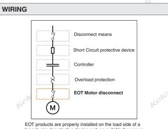
branch circuit protective device and are suitable for use as motor disconnects as illustrated above.
